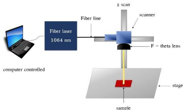
Figure 1: Experimental setup for paint removal using the fiber laser.
