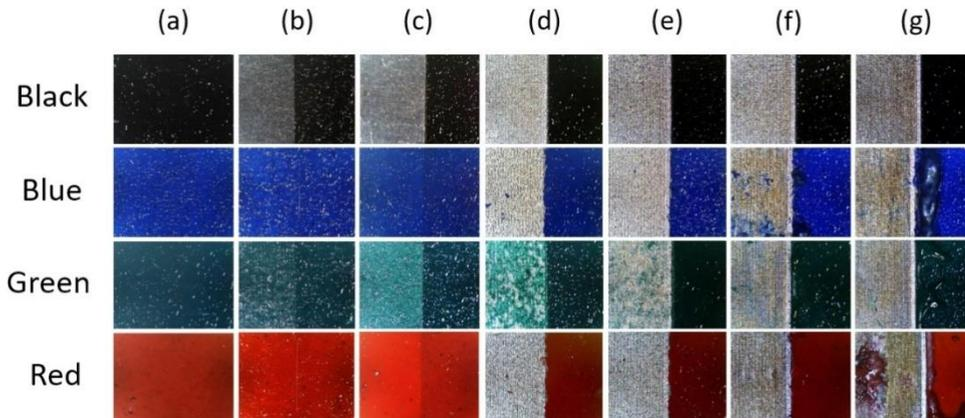
**Figure 3:** Microscope image of the removal of the averaged paint thicknesses of 30 microns using the fiber laser at the fluencies (b)  $0.15 \text{ J/cm}^2$ , (c)  $0.30 \text{ J/cm}^2$ , (d)  $0.60 \text{ J/cm}^2$ , (e)  $0.90 \text{ J/cm}^2$ , (f)  $1.20 \text{ J/cm}^2$  and (g)  $1.50 \text{ J/cm}^2$ . The column (a) shows the examples of painted surfaces before the removal by laser radiation.
