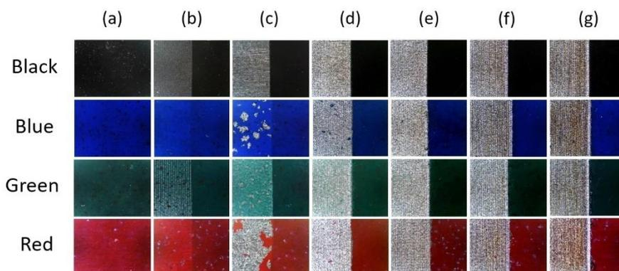
Figure 2: Microscope image of the removal of the averaged paint thicknesses of 10 microns using the fiber laser at the fluences (b)  $0.15 \text{ J/cm}^2$ , (c)  $0.30 \text{ J/cm}^2$ , (d)  $0.60 \text{ J/cm}^2$ , (e)  $0.90 \text{ J/cm}^2$ , (f)  $1.20 \text{ J/cm}^2$  and (g)  $1.50 \text{ J/cm}^2$ . The column (a) shows the examples of painted surfaces before the treat of laser radiation.
