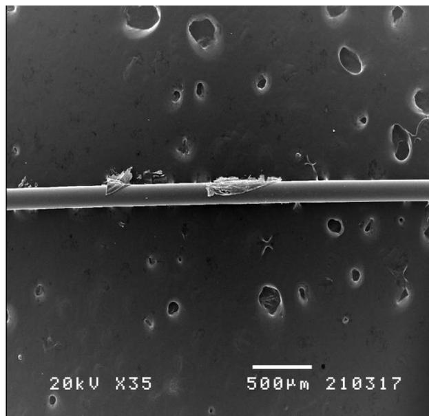
Figure 4: SEM image of an area of the wire cleaned by Q-switch radiation at  $1 \text{ Jcm}^{-2}$ .
