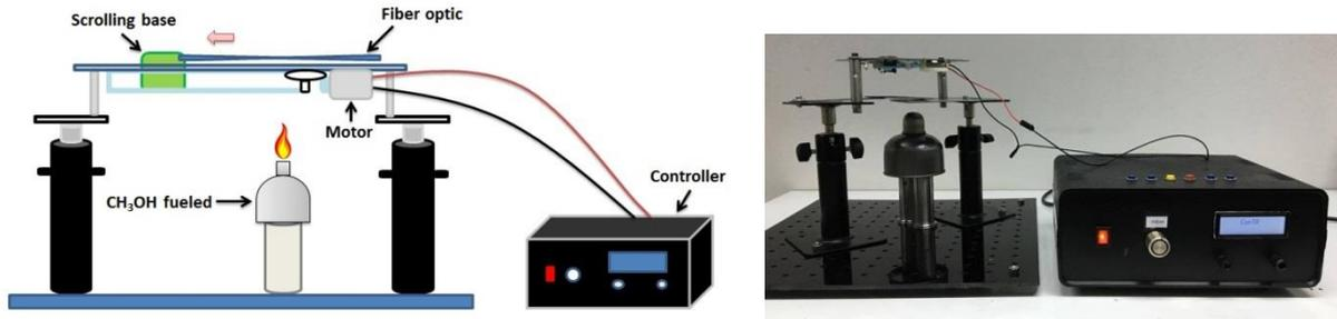
Figure 1: Schematic diagram of the automatic-controlled fiber drawing process.
